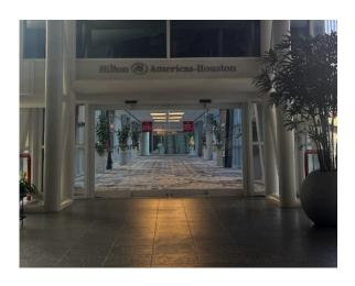
The convention center is connected to the hotel with an internal accessible path that features sufficient width, firm, stable and slip resistant surface and clear contrasted signage
